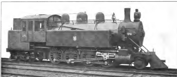
Fig. 46. Eight-Coupled (2-8-4) Tank Locomotive. Built by the American Locomotive Co. for the Dominion Coal Co. Cylinders 22 in. x 28 in., Working Steam Pressure 200 lbs. per sq. in., Heating Surface 2,687.47 sq. ft., Diameter of Drivers 55 in., Weight on Drivers 170,000 lbs., Total Weight 239,000 lbs.
